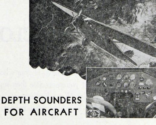
WITH the application of electricity to aircraft instruments, another chapter was written in the annals of air transportation. To-day's ship is not only swifter but safer and more dependable. Modern depth-sounding devices indicate instantly the height of the ship above the ground surface. A unique feature of General Electric's recently purchased monoplane is the almost completely electrified instrument panel.
