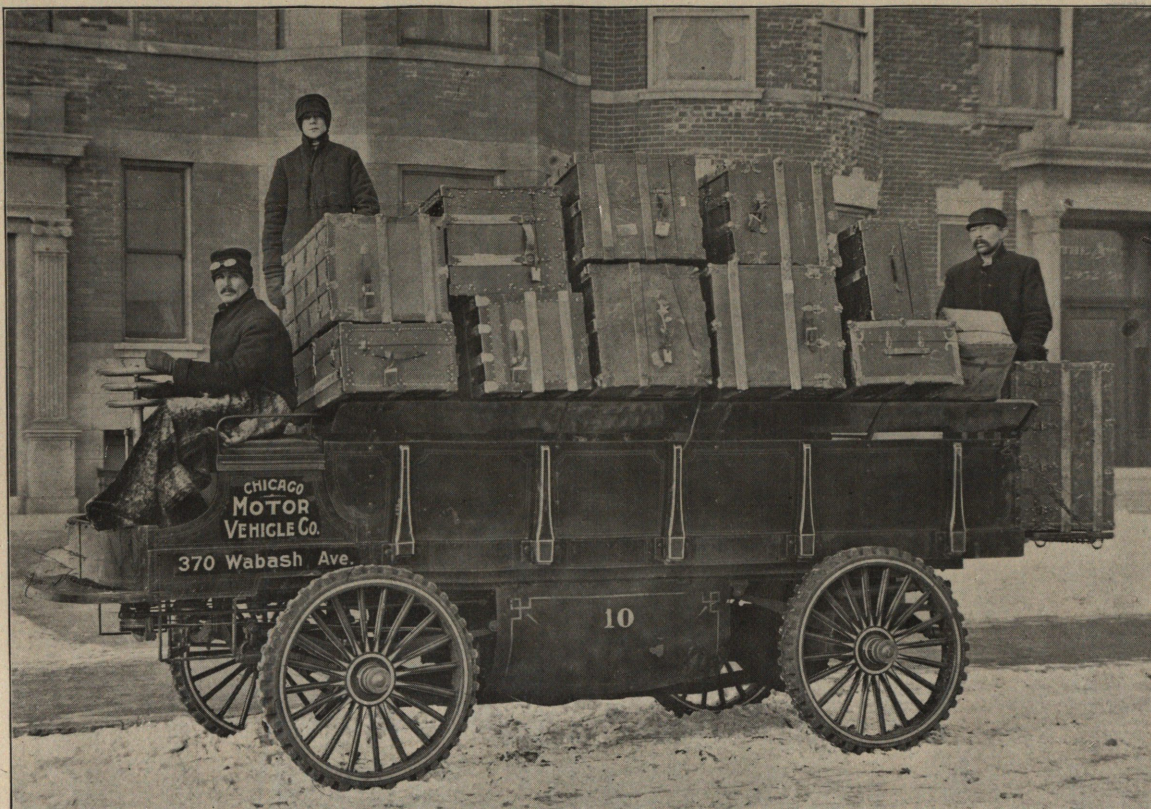
AUTO TRUCK WITH FROM 2 TO 4 TONS CAPACITY FURNISHED WITH ENCLOSED VESTIBULE FRONT
