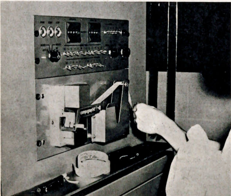
One of the compugraphic operators feeds the pre-typed tape into the newly acquired press computer.
