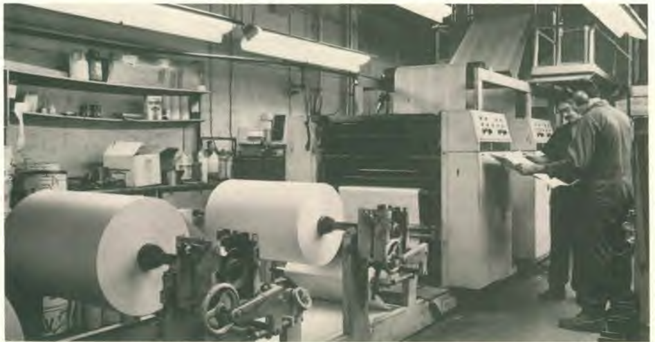
At Maracle Press in Oshawa huge rolls of paper feed the Web which prints and folds 20,000 signatures of Great Controversy an hour. Pressmen Bruce Adams and David Newman keep check on the printed sheets.
