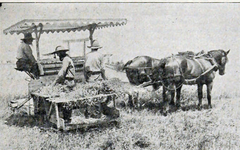
The McCormick Harvester of the Marsh type as it appeared in 1878. This type of machine was built in McCormick's Reaper factory in Chicago from 1875 to 1883. An elevator delivered the cut grain to a platform on the side of the machine where it was bound into bundles by hand. Two men could bind the grain as fast as it was cut. With the reapers of earlier years, a crew of four or five men was required to do the binding.
